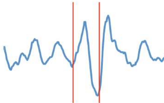
Figure 8: Detection of Pothole using algorithm STDEV(Z). Events are represented by measurements with standard deviation value above specific threshold level.
